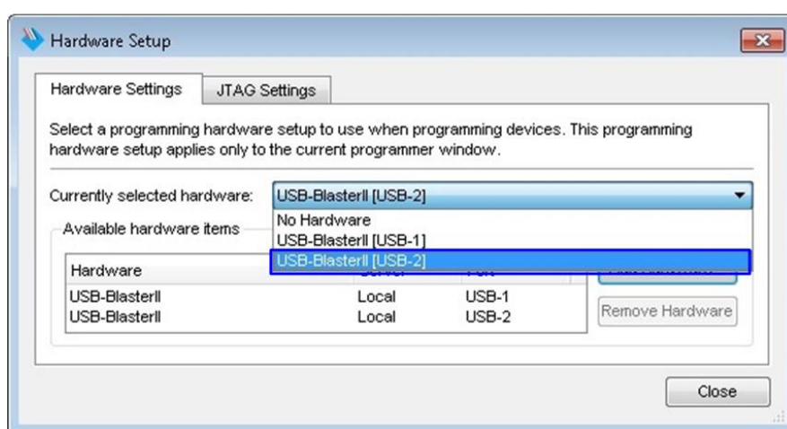
Figure 3-2 Two USB-Blaster cables when connecting two FPGA boards to PC
