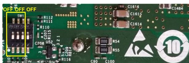
Figure 2-7 SW1 setting on Agilex F-series board
