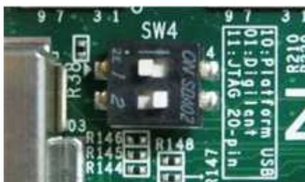
Figure 3-3 SW4 setting to use USB-to-JTAG on ZC706 board
