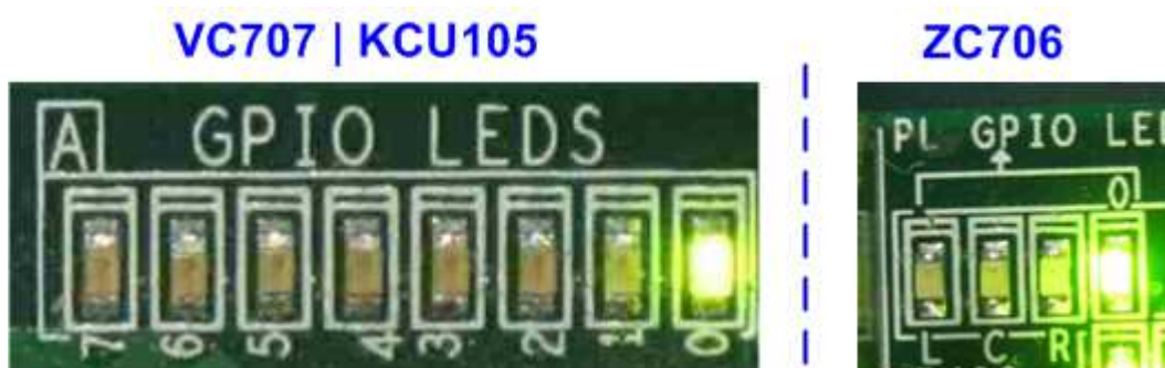
Figure 3-8 LED Status after push StartSW
