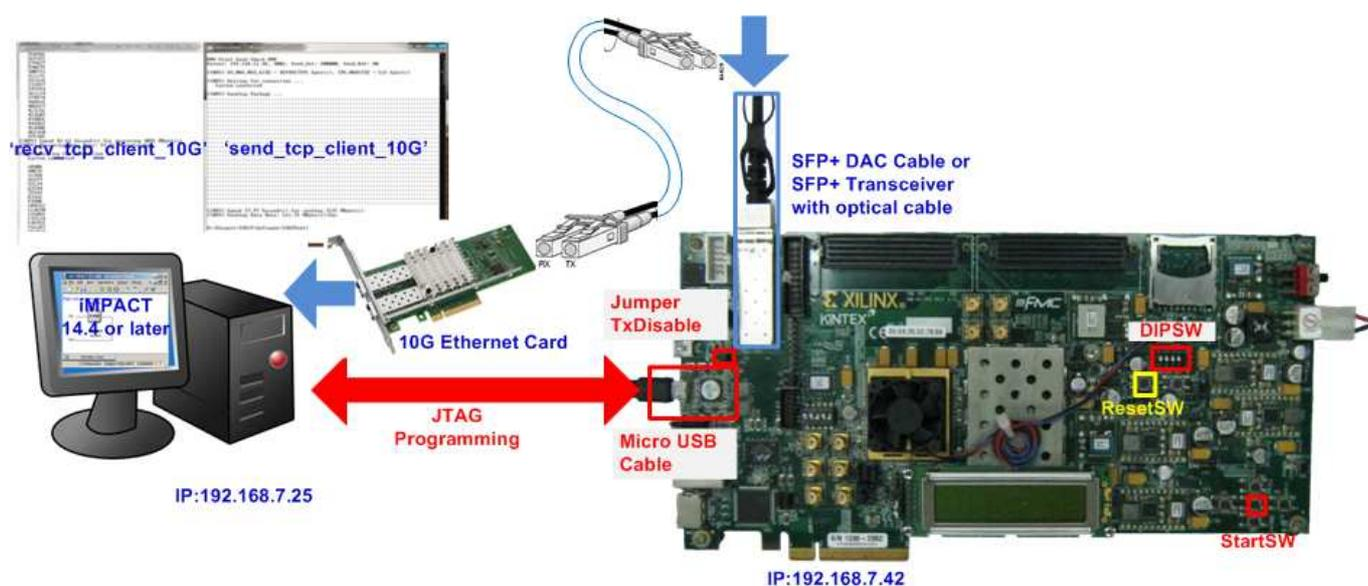
Figure 2 TOE10GIP Demo on Development board
