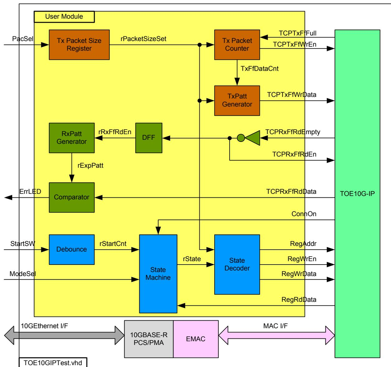
Figure 4 User Module and Test System block diagram
