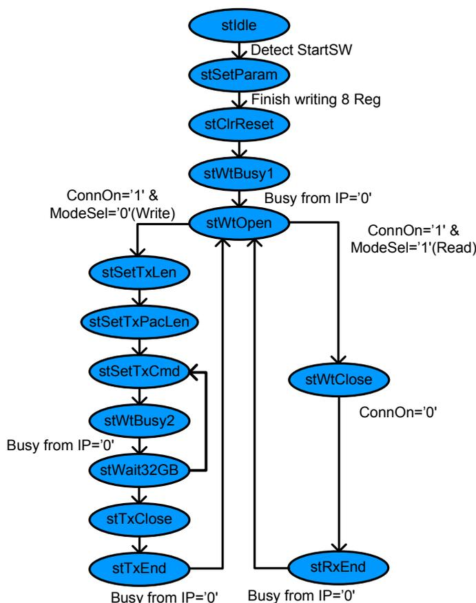
Figure 5 State Machine Diagram within User Module
