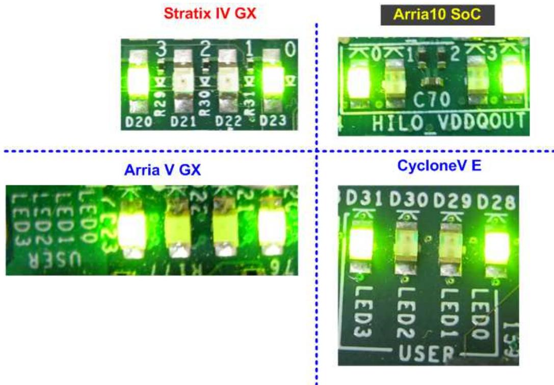
Figure 4-5 LED Status when running full duplex Demo for both modes
