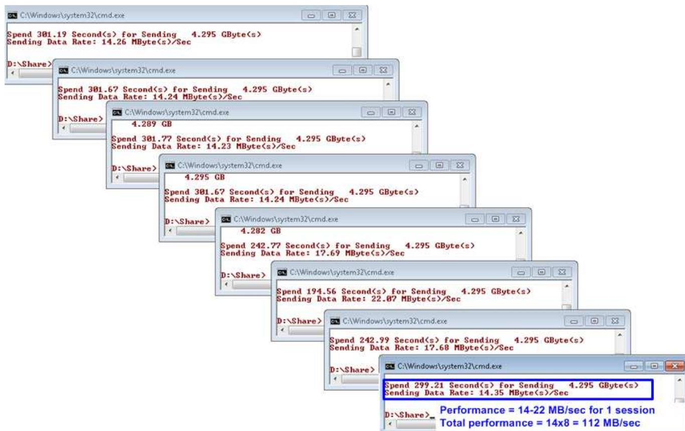
Figure 4-6 Performance when run receive data test using 8 sessions at the same time
