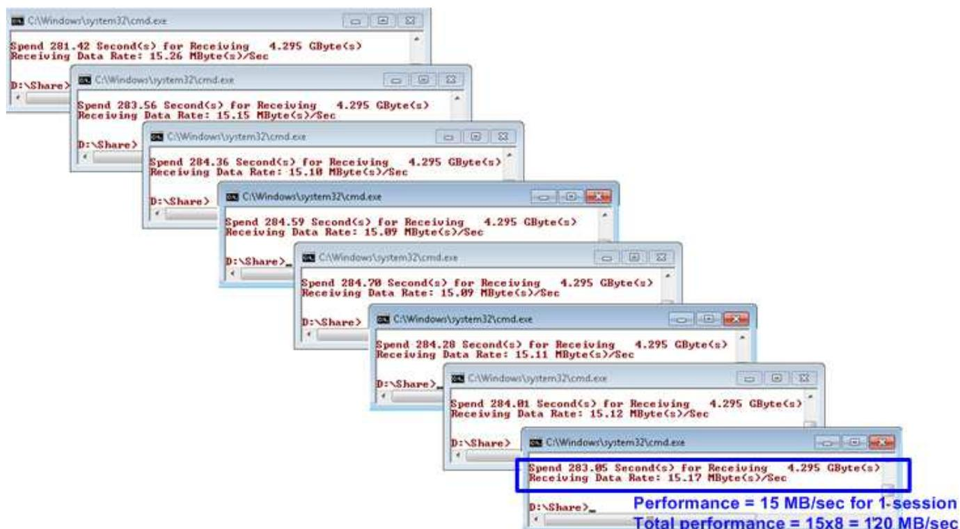
Figure 4-3 Performance when run send data test using 8 sessions at the same time
