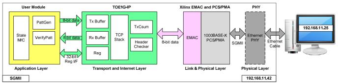
Figure 3 Hardware Architecture in FPGA board by SGMII (VC707/Zyng Mini-ITX)
