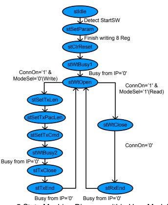
Figure 5 State Machine Diagram within User Module
