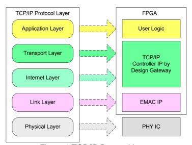
Figure 1 TCP/IP Protocol Layer
