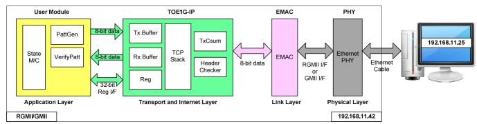
Figure 2 Hardware Architecture in FPGA board by RGMII or GMII (AC701/KC705)
