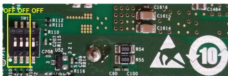
Figure 2-6 SW1 setting on Agilex 7 F-series board
