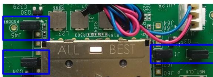
Figure 2-5 Set SFP[0]-[3] TX DISABLE for ZCU102
