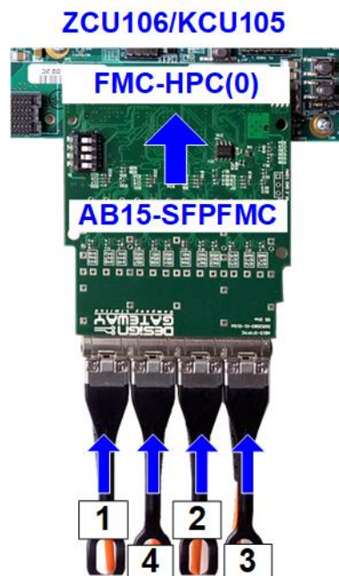
Figure 2-7 Four SFP+ cables connecting to ZCU106/KCU105 board
